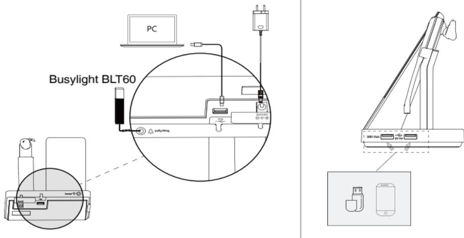
**Note:** Please make sure you connect the base to a DC power supply, not just the USB power supply. The included USB-A to USB-C cable cannot be used to connect other devices (for example, mobile device) to the USB hub port.
